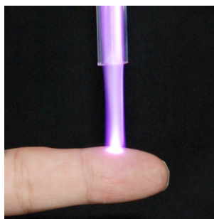
Fig. 2 LF (low frequency) plasma jet exhausted to a finger without burning.
